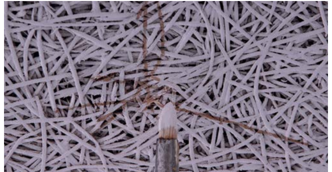
Chipped fibre: Cover chipped fibre with a fine brush or a spray gun using the supplied paint or an equivalent.
