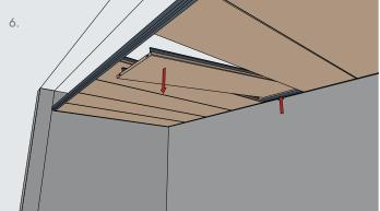
$\mathsf{HERADESIGN}\xspace$  Corridor elements are demountable by gently lifting the tile up and moving to the side.
