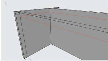
Mark the height on all perimeter walls (upper edge of the perimeter angle).
