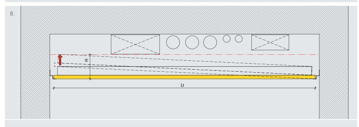
HERADESIGN® Corridor can be installed or demounted by gently lifting the tile and moving it to the side. The minimum installation height (H) is 150mm.
