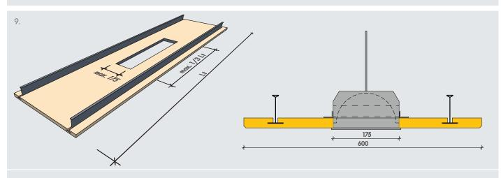
Additional loads >1.5 kg should be fixed to the soffit with independent hangers. For installations such as recessed lighting, loudspeakers etc., the maximum width of the cut-out opening is 175 mm. The maximum length of the cut-out opening is one third of the tile length (=1/3 Lt).
