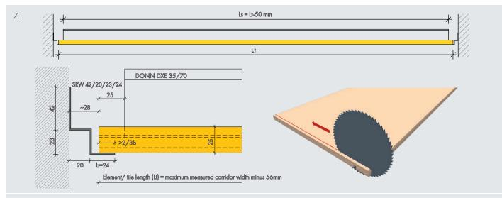
HERADESIGN<sup>®</sup> Corridor is available to order in every required length up to a maximum tile length (Lt) of 2400mm. To allow for structural tolerances, the main profiles are 25mm shorter than the tile, at both ends. The elements can be shortened by up to 50mm when required. This can be carried out with a hand saw, circular saw or with a table saw.
