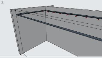
Install the perimeter angle using approved plugs and screws. Maximum spacing of the fixings 400mm. The perimeter angle should be mitred at the corners.
