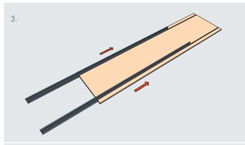
Push the T-profiles into the grooves on the reverse side of the HERADESIGN® Corridor panel. Centre the profiles. Tile overhang 25mm right and left.
